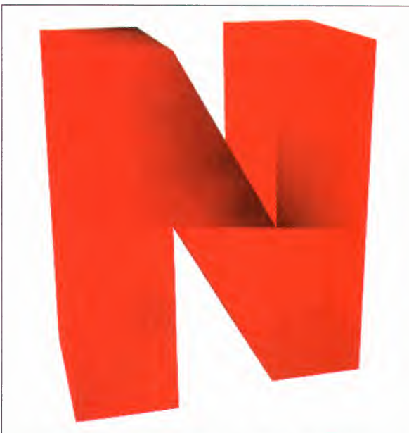
Using non-planar polygons will result in rendering errors like this. Converting everything to triangles will prevent it.
